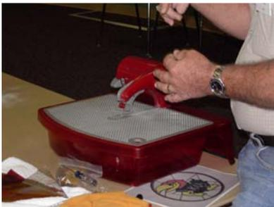
**The Band Saw:** Paul says the problems with the band saw are that the top plate fills up with dust and makes a mess, no water containment when it's running, water shoots out, it is hard to clean, if you forget to turn the water flow off it can overflow, and the metal parts rust. It is good for cutting heavier pieces of glass and you can get a finer cut than with the ring saw. The band saw is good for deep inside cuts and smaller cuts. It is also much quieter than the ring saw.
